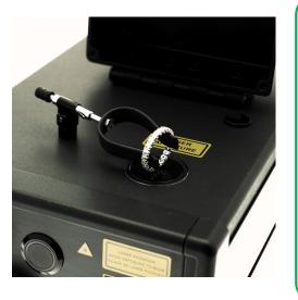
No sample preparation needed. GemmoRaman-532 works on polished, rough and mounted gems. The right image shows the magnetic ring clip accessory in use.
